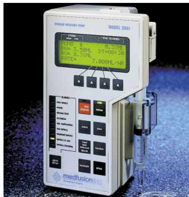
Figure 3-11 Syringe infusion pump for the administration of small amounts of medication. (Courtesy of Medex, Inc.)
